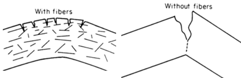
Fig. 1. Demonstration of how fibers prevent cracks in a brittle material from propagating through the fibers into their path
